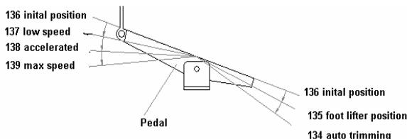
Fig. 4-1 pedal movement of each position parameter
