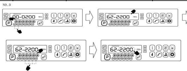
Step 4: the parameter confirms correct, press **P** key until the red light of HMI are bright or buzz produces a long loud, release **P** key, HMI and the whole system restore storage parameter.
