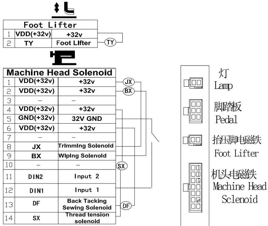
Fig. 4-1 controller link
