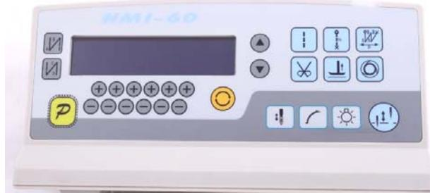
Step 1: First press **P** + **○**, LCD shows **PD 0000**, then press **P**, LCD shows **PD-0000**.
